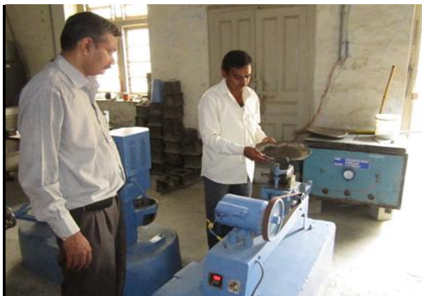
Fig 3: Set up of Vibrating Machine and Crucible for Mixing Cement and Fine Aggregate (Sand)
