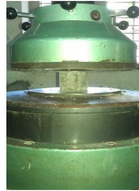
Fig 4: Set up of Compressive Testing Machine
