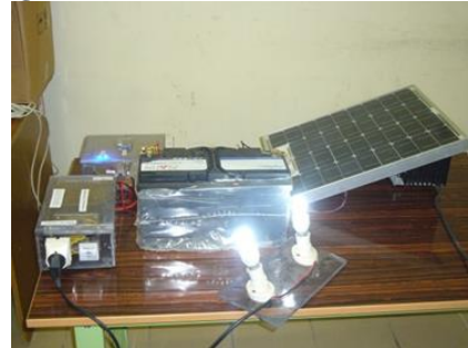
Figure 4d: The whole system during the test (battery, regulator, AC and DC lamps, DC/AC inverter)
