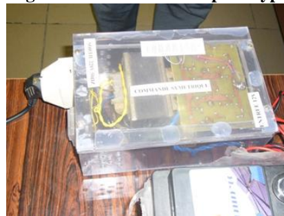
Figure 4c: The associated DC/AC inverter
