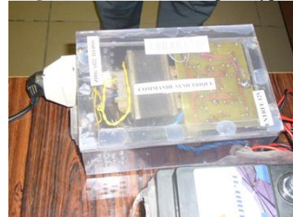
Figure 4c: The associated DC/AC inverter
