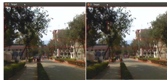
Fig.5 Moving Objects are detected using the background Subtraction method in different frames.
