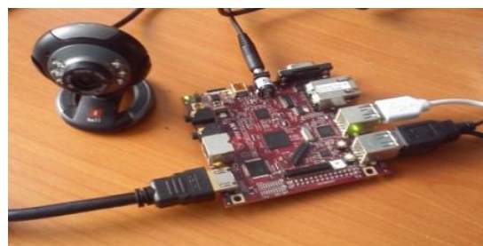
Fig.1. Experimental setup with Beagleboard and web camera
