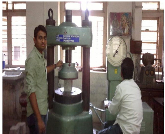
Figure: 4 Setup of Compression Strength Testing Machine
