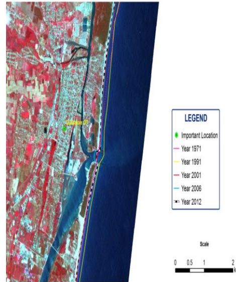
Fig. 6 Erosion/Accretion during 1971 to 2012 (Segment-B)
