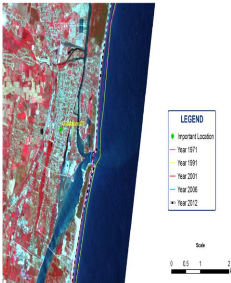
Fig. 6 Erosion/Accretion during 1971 to 2012 (Segment-B)
