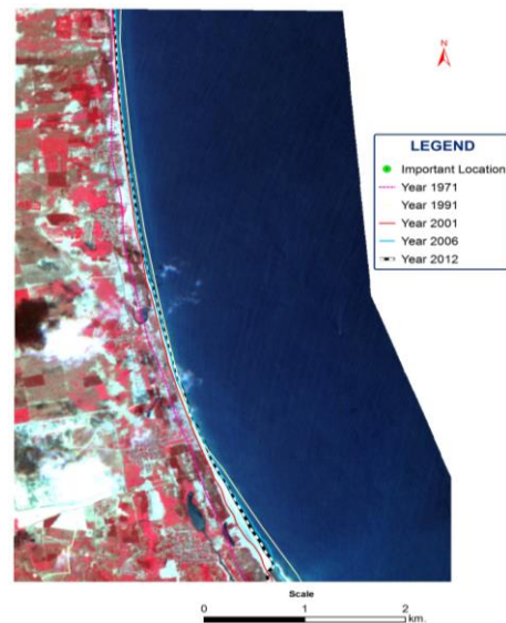
Fig. 8 Erosion/Accretion at segment-D during 1971 to 2012
