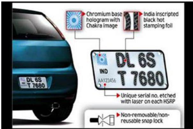
Fig 2.1: High Security Number Plate Description [2].
