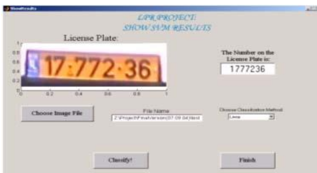
Fig 3.3: GUI for identifying number on a license plate using SVM classifier.
