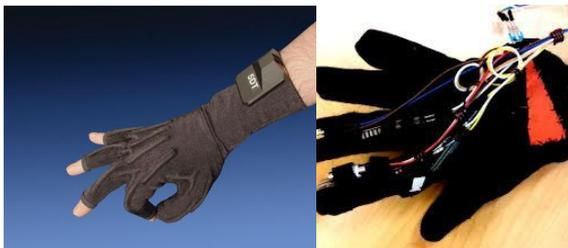
Figure 3 Glove Based Hand Gesture Recognition [9]
