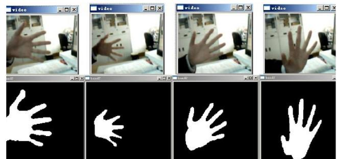
Figure 1 Hand Gesture Recognition in Rotation State [13]
