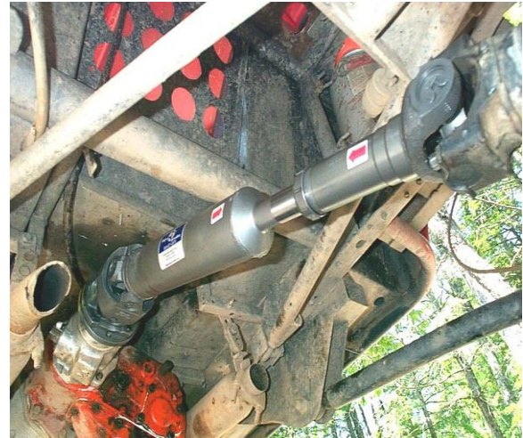
Fig 5: A two-section drive shaft of a truck.
