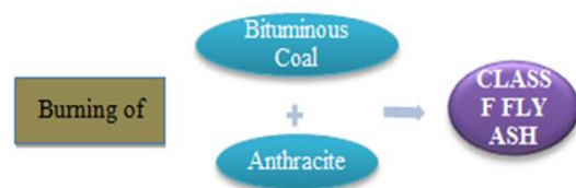
Figure 1 : Production of Class F Fly ash
