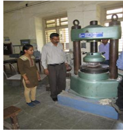
Figure: 7 Setup of Compression strength test machine
