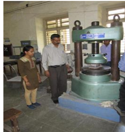
Figure: 7Setup of Compression strengthtest machine TABLE -6 COMPRESSIVE STRENGTH OF BRICKS (230X115X75) AT 7, 14, 21DAYS FOR STONE WASTE FLY ASH BRICKS
