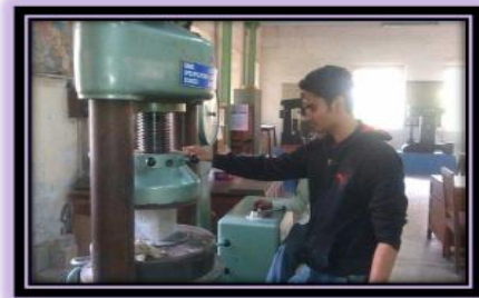
Figure: 6 Setup of Compression Strength Testing Machine Table -7 Compressive Strength Of Cubes(150x150x150)For M25 Mix At 7, 14, 28 Days
