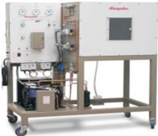
Figure 1a: Advanced Commercial Refrigeration Trainer (overview)
