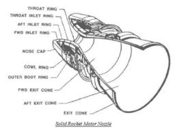
Fig.-2: Solid Rocket Motor Nozzle
