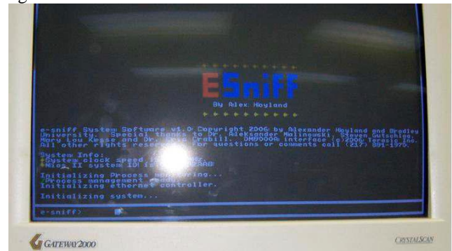
Fig. 5 - Typical screenshot of the VGA controller output. The status line is the portion that reads "Initializing system." Above this is the output section, and at the bottom is the keyboard input line, which contains the "e-sniff>" prompt.
