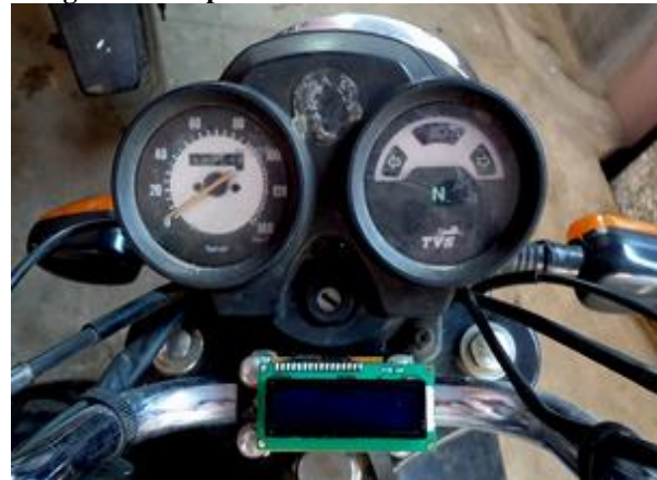
Figure 6. LCD mounted near the existing dashboard
