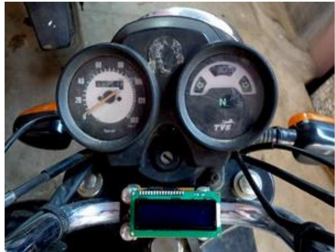
Figure 6. LCD mounted near the existing dashboard
