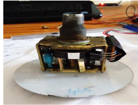
Figure 5. Optical sensor attached to odometer
