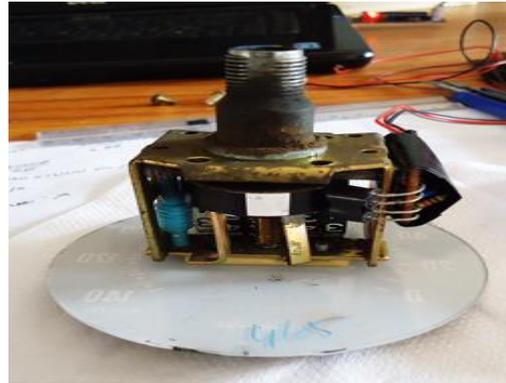
Figure 5. Optical sensor attached to odometer
