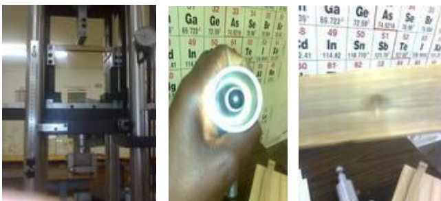
Fig 4:3 spherical ball pressing the work Fig 4:4 spherical ball fig 4:5 result of worked piece
