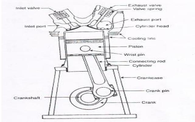
Fig. Air-cooled I.C. engine
