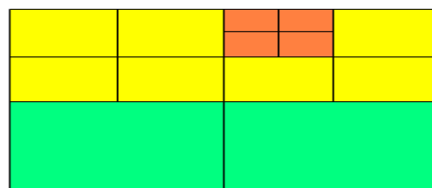
Figure 1: Green color represents 16 x 16 block. Yellow color represents 8 x 8 block. Orange color represents 4 x 4 block
