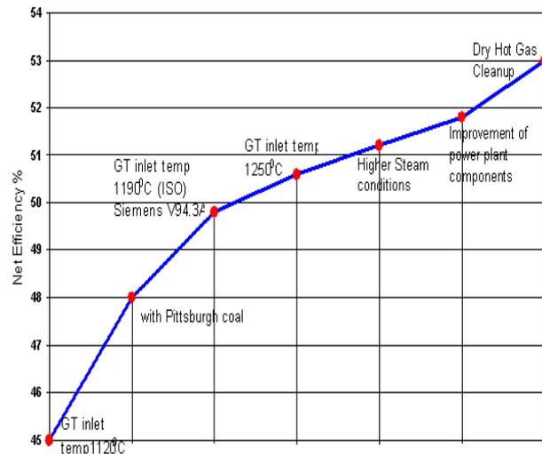
Fig 2 Expected Improvement of IGCC Power Plant Efficiency
