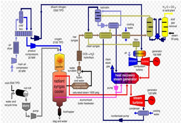
**Fig 1 Integrated Gasification Combined Cycle (IGCC) Power Plant**
