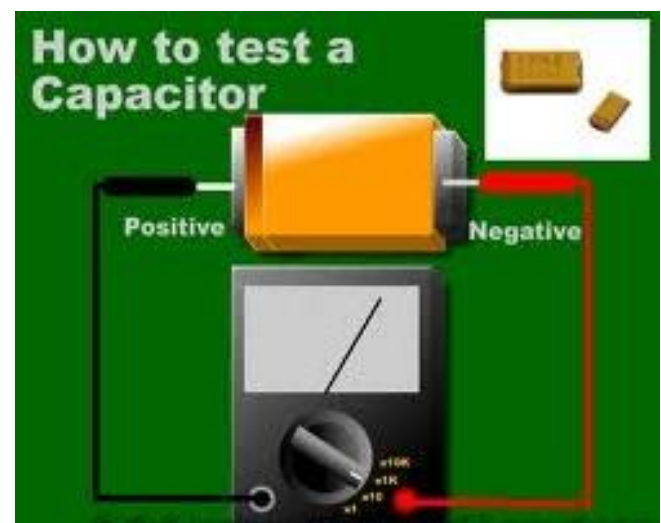
Fig1: capacitor testing using multimeter
