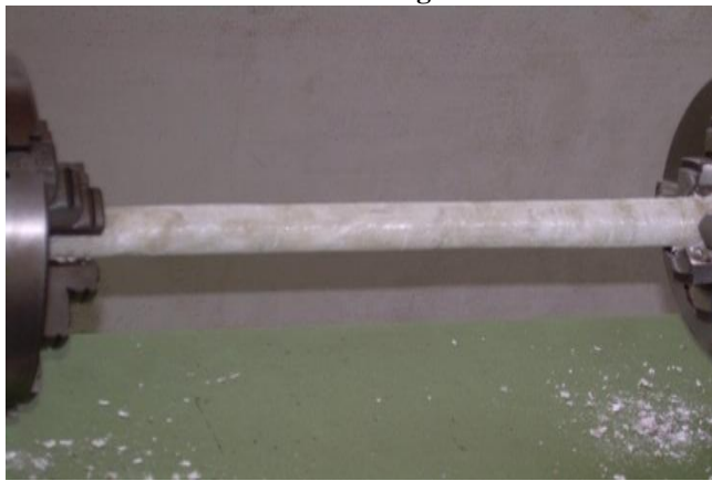
b) Delamination of composite layers from the aluminum tube
