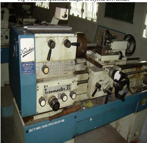
Fig 5 Lathe machine used to cut the specimen ends to its final dimensions
