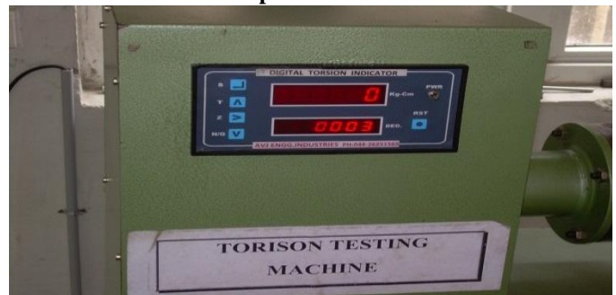
Fig 7 Digital Torsion Indicator image on Torsion Testing machine
