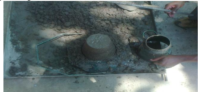
Picture showing the cone of the workability test
