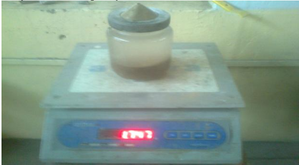
Picture showing the pycnometer with quarry dust, water
