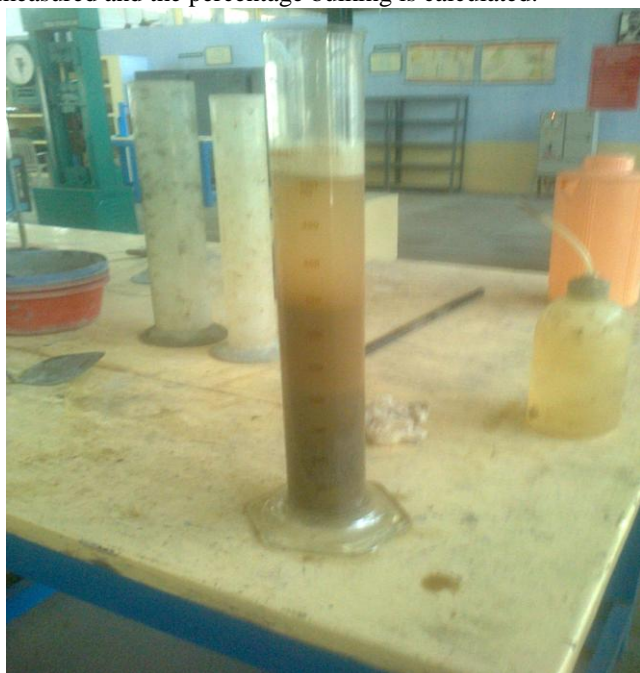
Picture showing the test for the bulking of quarry dust
