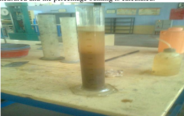
Picture showing the test for the bulking of quarry dust
