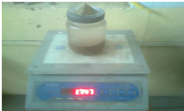
Picture showing the pycnometer with quarry dust, water
