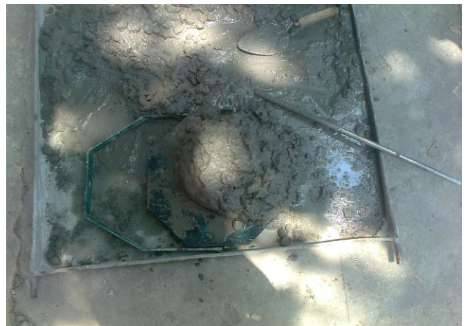
Picture showing the complete failure of the slump cone at maximum water-cement ratio
