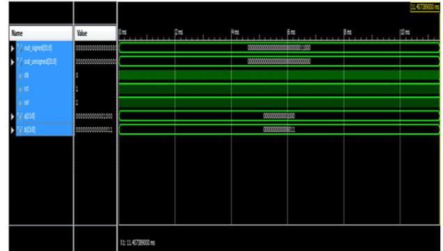
Figure 8: For signed-unsigned Booth Multiplier where a=8 and b=3 sel=0(unsigned multiplier is chosen)
