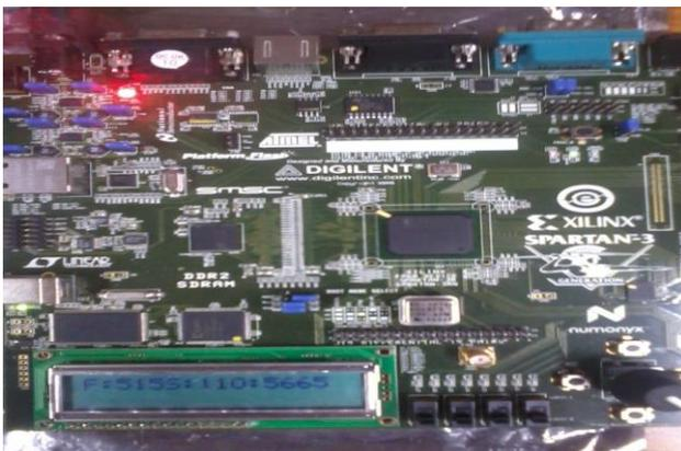
**Figure 13:FPGA implementation of Booth's multiplier**
