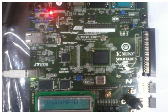
Figure 14:FPGA implementation of Baugh-wooley multiplier
