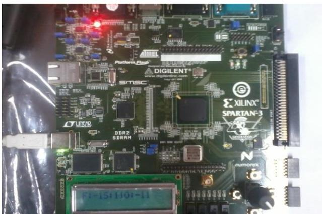
**Figure 14:FPGA implementation of Baugh-wooley multiplier**
