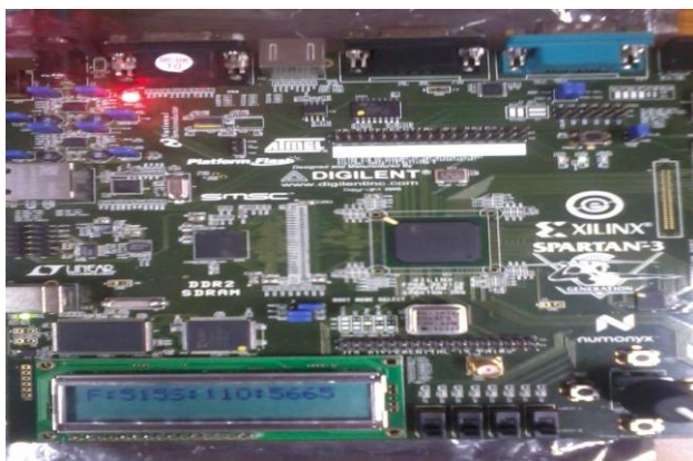
Figure 13:FPGA implementation of Booth's multiplier
