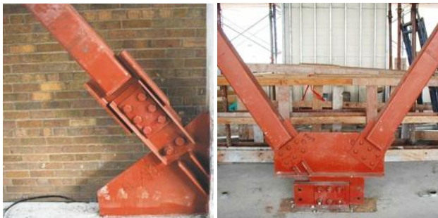
Figure 2. Friction damper in single diagonal bracing Figure 3. Friction damper in chevron bracing (inverted)
