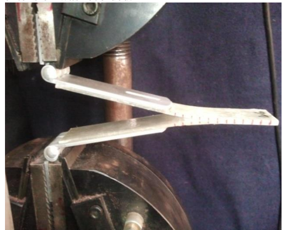
Fig 1b: Crack propagation in glass-epoxy composite under DCB test
