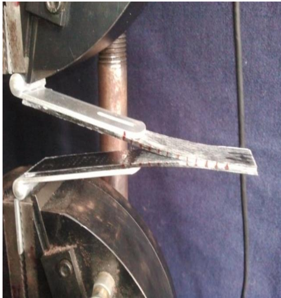
Fig 1c: Crack propagation in glass-carbon hybrid composite under DCB test
