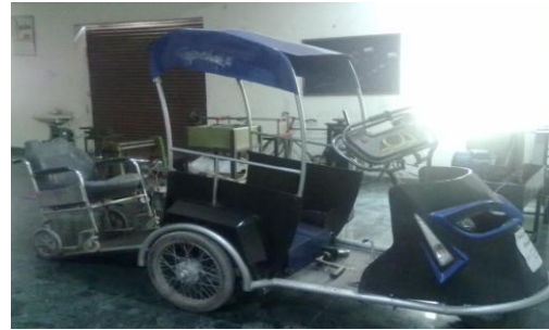
Fig8, special designed wheel chair which can be set in the electro handy and can be used as seat of electro handy
