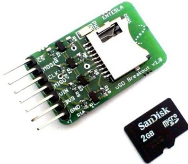
Figure 7: SD card and reader.
