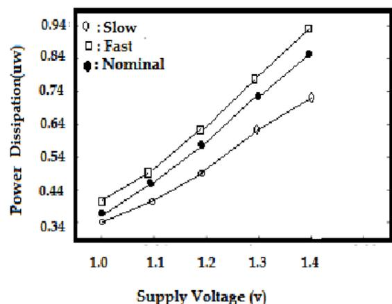
Figure 6.Measurement of power dissipation at various supply voltages at 2 MHz frequency.
