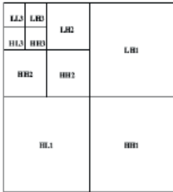
Figure 3: Three Level Wavelet transform.
