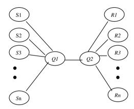
S1,S2,,R1and R2 have bandwidth of 2Mb and delay of 10 ms S3 to Sn and R1 to Rn have bandwidth of 10Mb S3 to Sn and R3 to Rn have delay from 14 to 15 ms Q1 to Q2 have 20ms delay and bandwidth 0.7Mb
