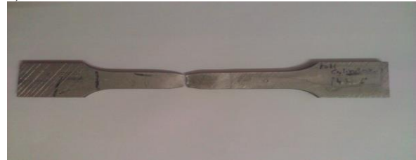
Figure-4- Failure of Welded Specimen in Tensile Test (Single pass Cylindrical)
