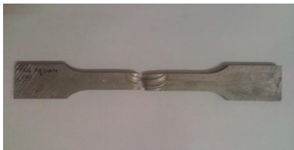
Fig-8- Failure of Welded Specimen in Tensile Test (Single pass Square)
