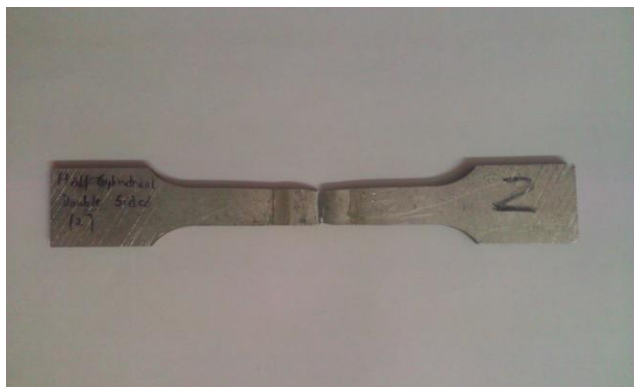
Fig-6- Failure of Welded Specimen in Tensile Test (Double pass Cylindrical)
