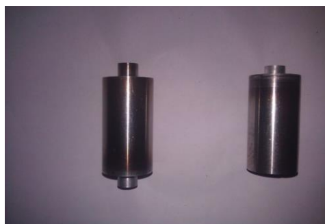
Fig-2 a) Circular Tool Profile
