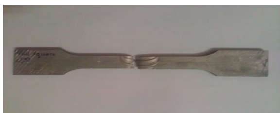
Fig-8- Failure of Welded Specimen in Tensile Test (Single pass Square)
