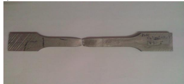
Figure-4- Failure of Welded Specimen in Tensile Test (Single pass Cylindrical)
