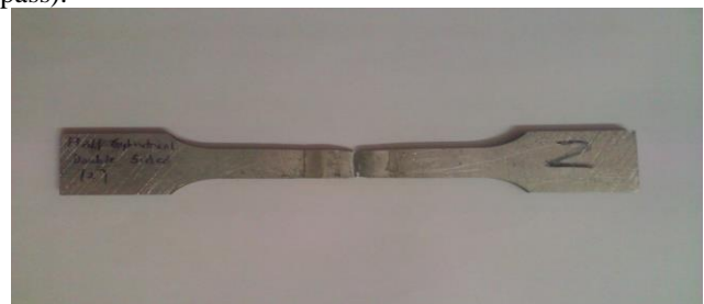
Fig-6- Failure of Welded Specimen in Tensile Test (Double pass Cylindrical)
