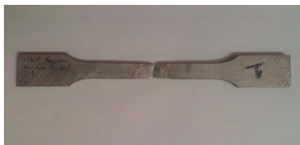
Fig-10- Failure of Welded Specimen in Tensile Test (Double pass Square)
