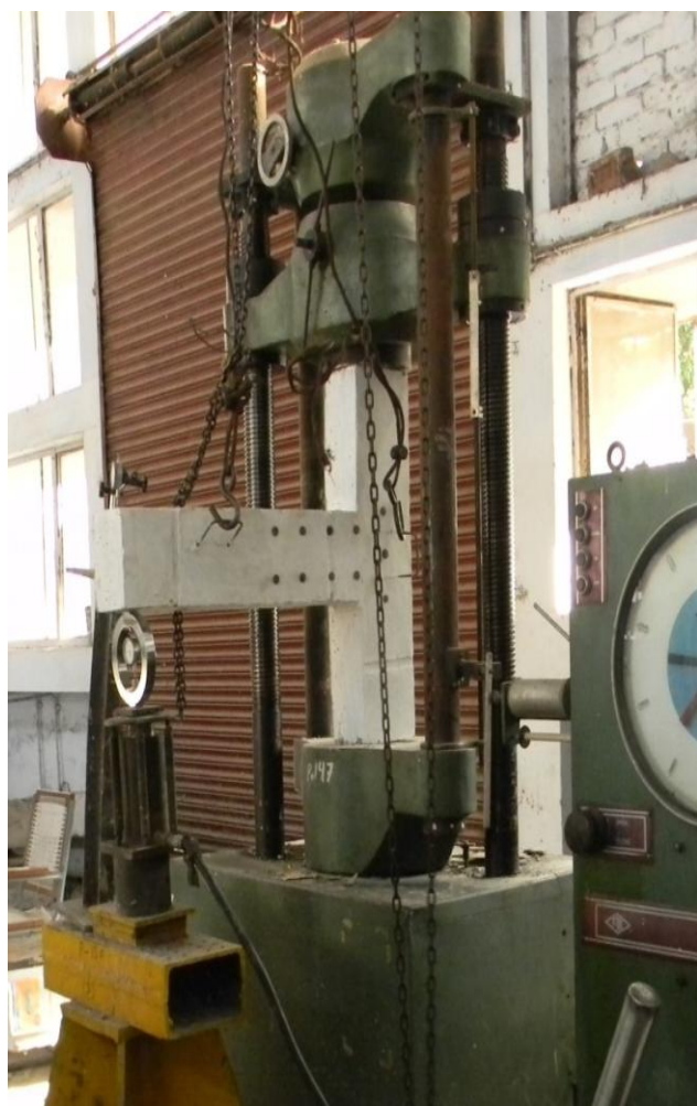
Figure 1.4 Confinement of a Beam-Column joint
