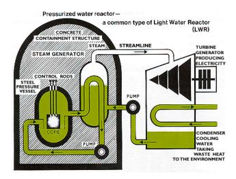
A PWR has fuel assemblies of 200-300 rods each, arranged vertically in the core, and a large reactor would have about 150-250 fuel assemblies with 80-100 tonnes of uranium.
