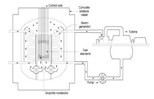
The AGR was developed from the Magnox reactor, also graphite moderated and CO2 cooled, and one of these is still operating in UK to late 2014. They use natural uranium fuel in metal form. Secondary coolant is water
