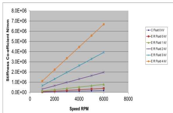
Fig: 8 Speed Vs Stiffness for  $e=0.5, L/D=0.4$
