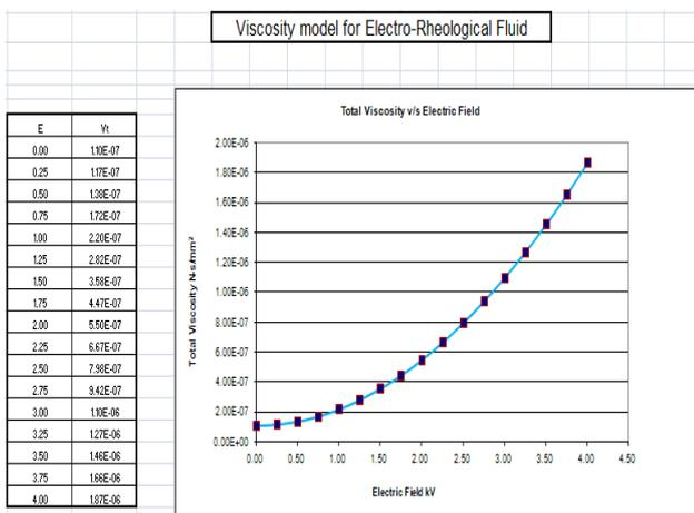
Fig: 4 - viscosity model for ER fluid
