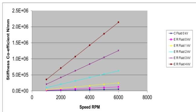
Fig: 7 Speed Vs Stiffness for  $e=0.25, L/D=0.4$
