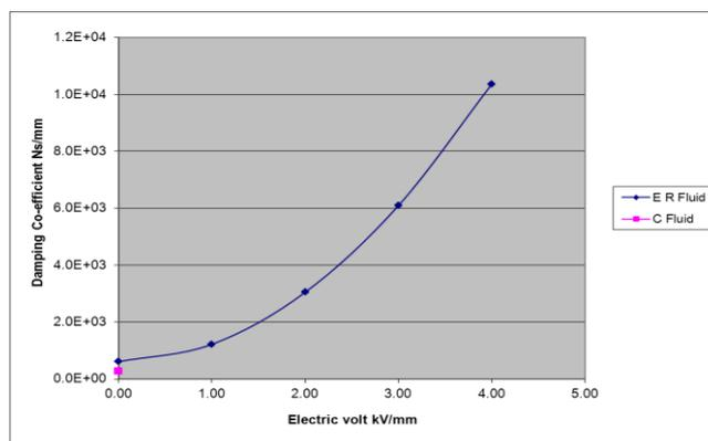
Fig: 11 Electric Current Vs Damping for  $e=0.25, L/D=0.4$
