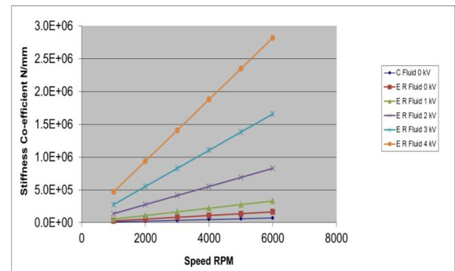
Fig: 6 Speed Vs Stiffness for e=0.5, L/D=0.3
