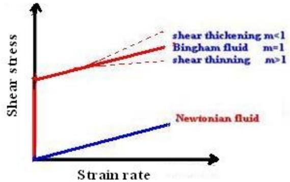
Fig: 3 -Visco-plasticityHerschel-Bulkley model
