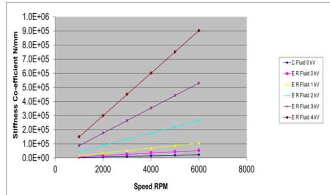
Fig: 5 Speed Vs Stiffness for e=0.25, L/D=0.3
