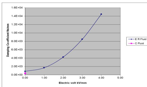
Fig: 12 Electric Current Vs Damping for  $e=0.5, L/D=0.4$
