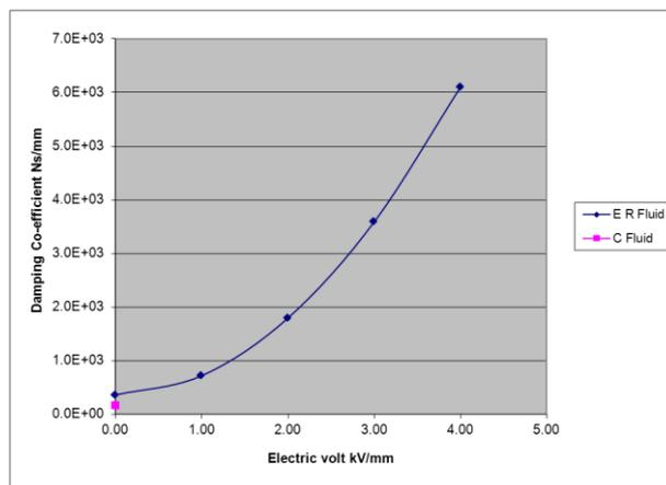
Fig: 10 Electric Current Vs Damping for  $e=0.5, L/D=0.3$
