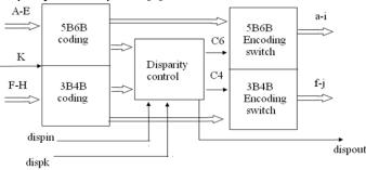
Figure.1: Block Diagram of Conventional 8B/10B Encoder
