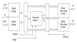
Figure.3: Block Diagram of pipelined 8B/10B Encoder Architecture
