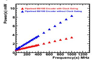
Figure: 9 Clock Power of Pipelined 8B/10B Encoder and Clock Gated Pipelined 8B/10B Encoder
