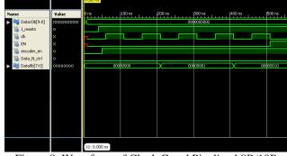
Figure.8: Waveform of Clock Gated Pipelined 8B/10B
