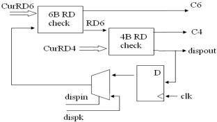
Figure.2: Block Diagram of Disparity Control
