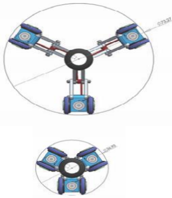
Fig.2 The range of the exterior diameter of the robot is 37mm~73mm.
