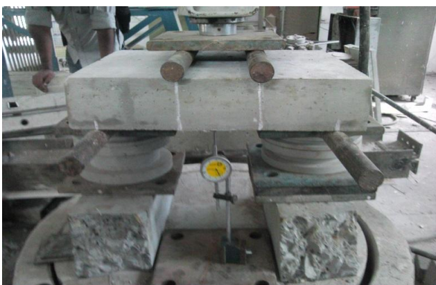
Figure (8) LWSP under flexural loading for testing purpose
