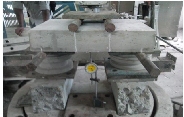
Figure (8) LWSP under flexural loading for testing purpose
