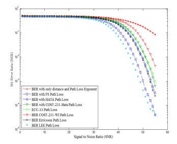
Fig. 3: BER vs SNR for PAFP using different path loss models
