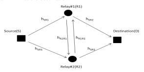
Fig. 1: Inter-relay communication using three time slot protocol
