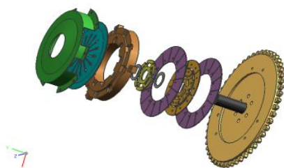
Figure.2 Exploded view of single plate clutch
