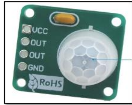
Figure (4) IR Motion sensor unit
