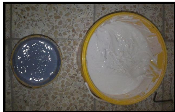
Figure (3) epoxy resin (A + B) .
