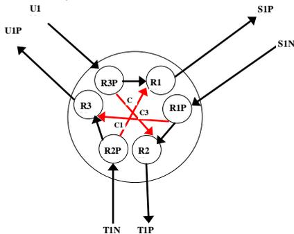
Fig-3: Three road crossing represented in a graph (Without a self right turn in the Crossing)
