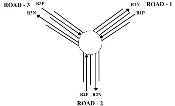
Fig 1: Streams of traffics of a three road junction
