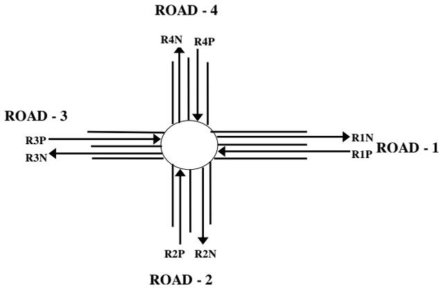
Fig 2: Streams of traffics of a four road Junction
