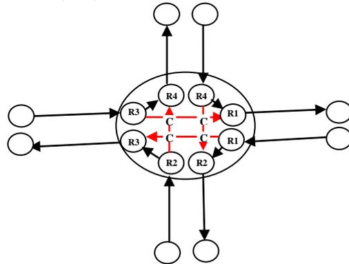
Fig-4: Four road crossing represented in a graph (Without a Self Right Turn in the Crossing)
