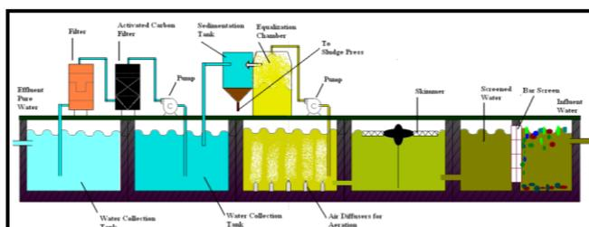
Figure 1: Components of the Waste Water Treatment Plant at site
