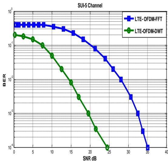
Fig .6. BER performance of LTE Transceiver based OFDM DWT in SUI-5 Channel
