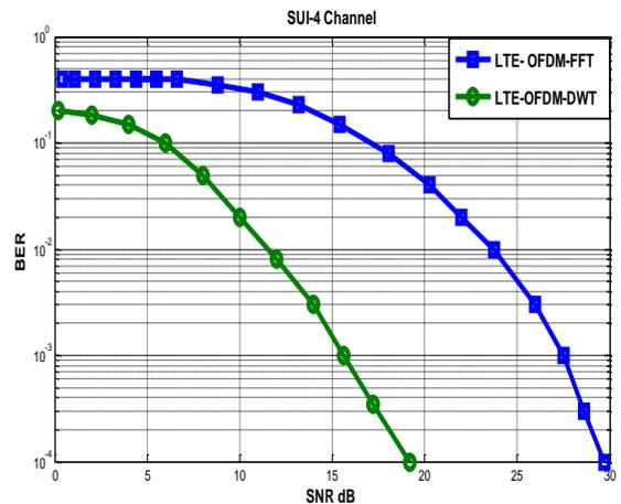
Fig. 5. BER performance of LTE Transceiver based OFDM DWT in SUI-4 Channel
