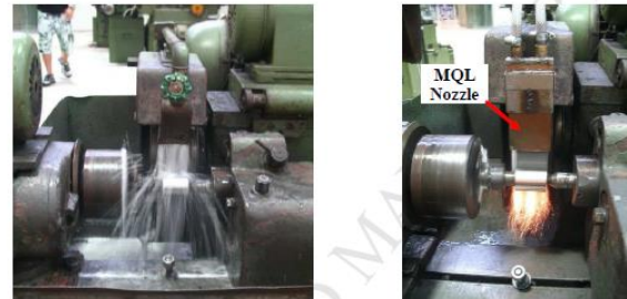
(a) Original nozzle of the grinding machine. (b) Nozzle used in the MQL experimentation
