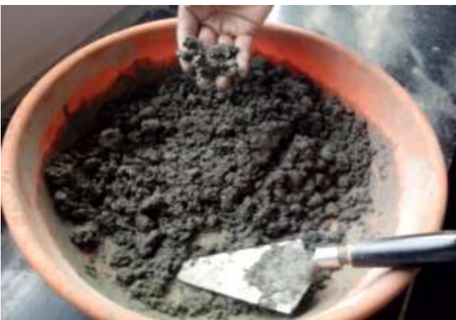
Image No.2 One Hour after Mixing Mortar
