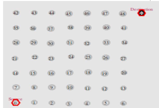
Fig. 5 Finding Shortest Path Nodes from Source to Destination Using AODV in NAM
