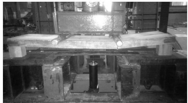
Fig. 4 Practical Test Set-Up IBS Walls
