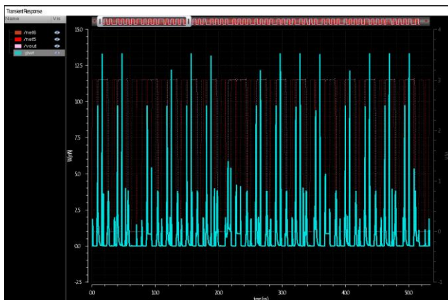
Fig. 14 Power Waveform of D flip-flop
