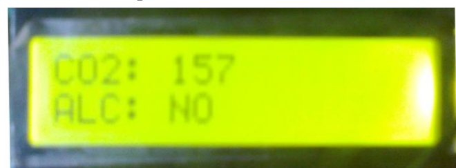
Fig -5: Display of CO 2 content and alcohol content
