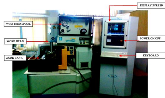
Fig. 2: Wire-cut EDM (ELEKTRA SPRINTCUT-734) of Electronica Machine Tools Ltd.
